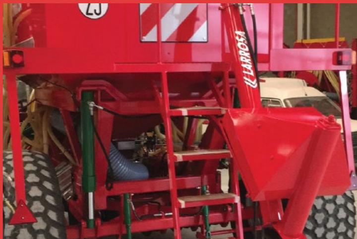
VIS SANS FIN ARRIERE REPLIABLE
